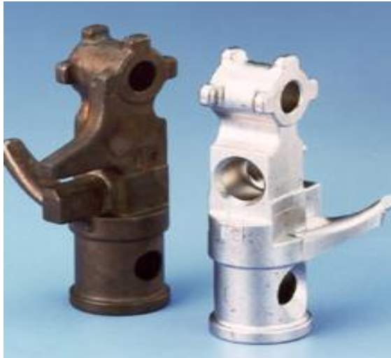
A collection of powder metallurgy parts.
