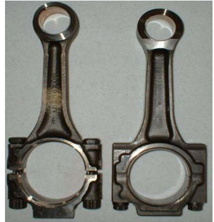
Connecting Rods: Forged on left; P/M on right
